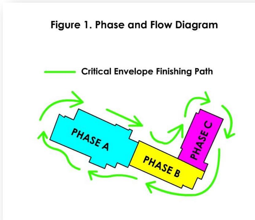
After analyzing the project schedule, it appears there may be an area for improvement when it comes to the sequence that the façade is installed. A potential solution to the schedule would be starting on a more critical corner of the building where site constraints may cause delays further in
